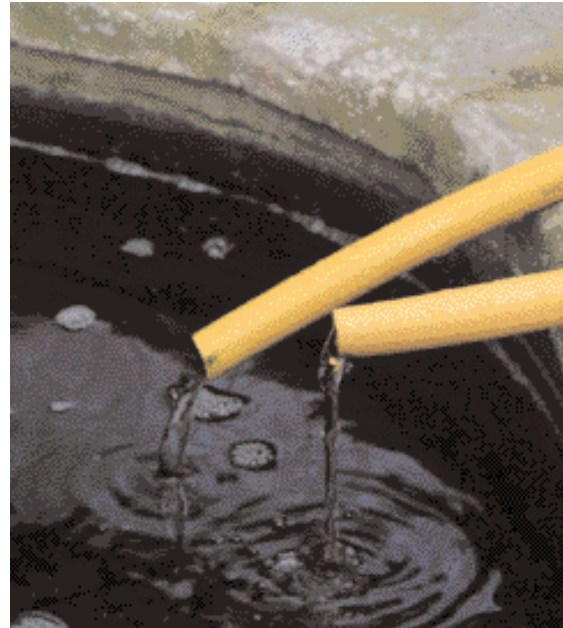
The water coming from the hose on the left is from an R/O plant and has a TDS of 5ppm, and KH of zero. The water from the hose on the right is mains water and has a TDS of about 300ppm, and a KH of about 11dH. But, the result of these mixing is a TDS of 75ppm, and KH of 2.75dH... that's more like it
