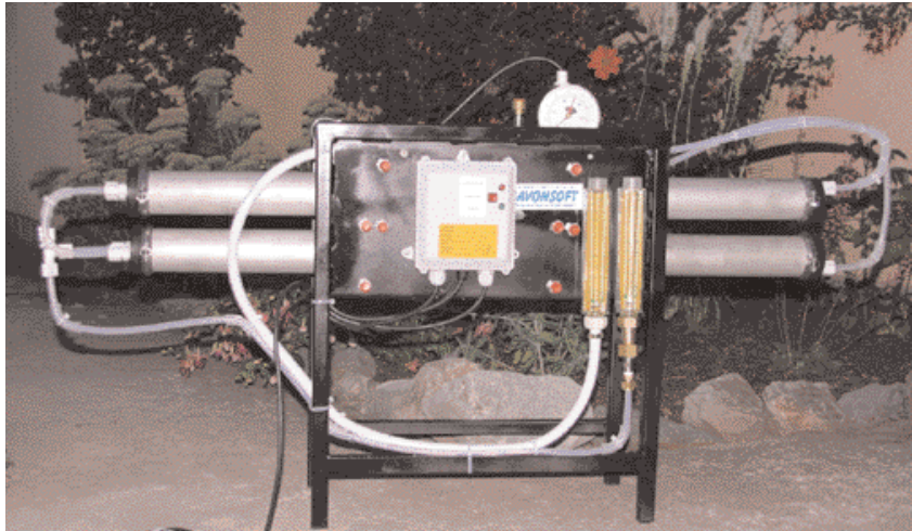
This particular R/O plant wastes very little water. But, RO water alone is dangerous, and must be mixed with mains water in order to obtain the kind of water you desire
