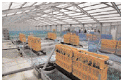
Momotaro Koi Farm use 'Bacteria House' media in these shower filters, partly to lower the total hardness of the water
