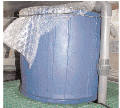
A 'Bacteria House' shower filter, which quite simply sits on top of the filter system. This is made from a plastic drum, which has a perforated base, thus allowing water to fall freely back into the main filter system. A pump pushes water up the grey pipe, and through the 'shower' holes, which then pours down over the filter media, and back into the main filter
